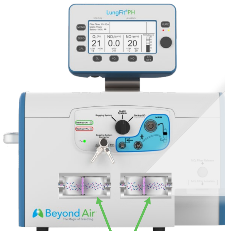
Main and Backup Ionizers
